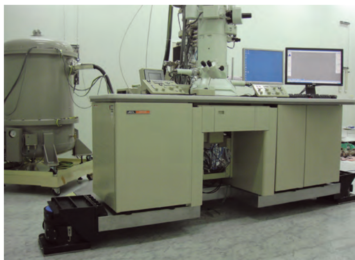
STACIS® 65 Series Floor Platform supporting a JEOL JEM-2100F Transmission Electron Microscope (TEM).
