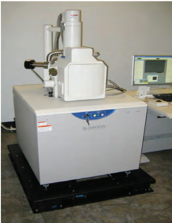
STACIS® iX SEM-Base™ Floor Platform isolating an FEI Helios NanoLab DualBeam SEM/FIB (top left), a JEOL JSM-6700F Field Emission Scanning Electron Microscope (top right), an Hitachi S-3400N SEM (bottom left), and a Field Emission Scanning Electron Microscope (bottom right).
