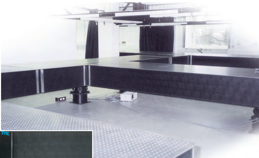
Precision-machined steel mating joiner plates are aligned and welded to multiple tops
