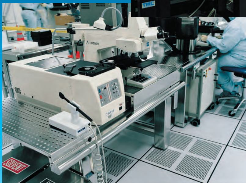
Custom electropolished stainless steel vibration isolation table installed at Motorola MOS-12. Photo courtesy of Motorola.
