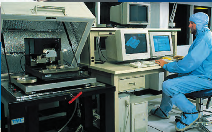
Integrated vibration isolation table/acoustic enclosure for Digital Instrument Atomic Force Microscope. Photo courtesy of Disc Manufacturing.
