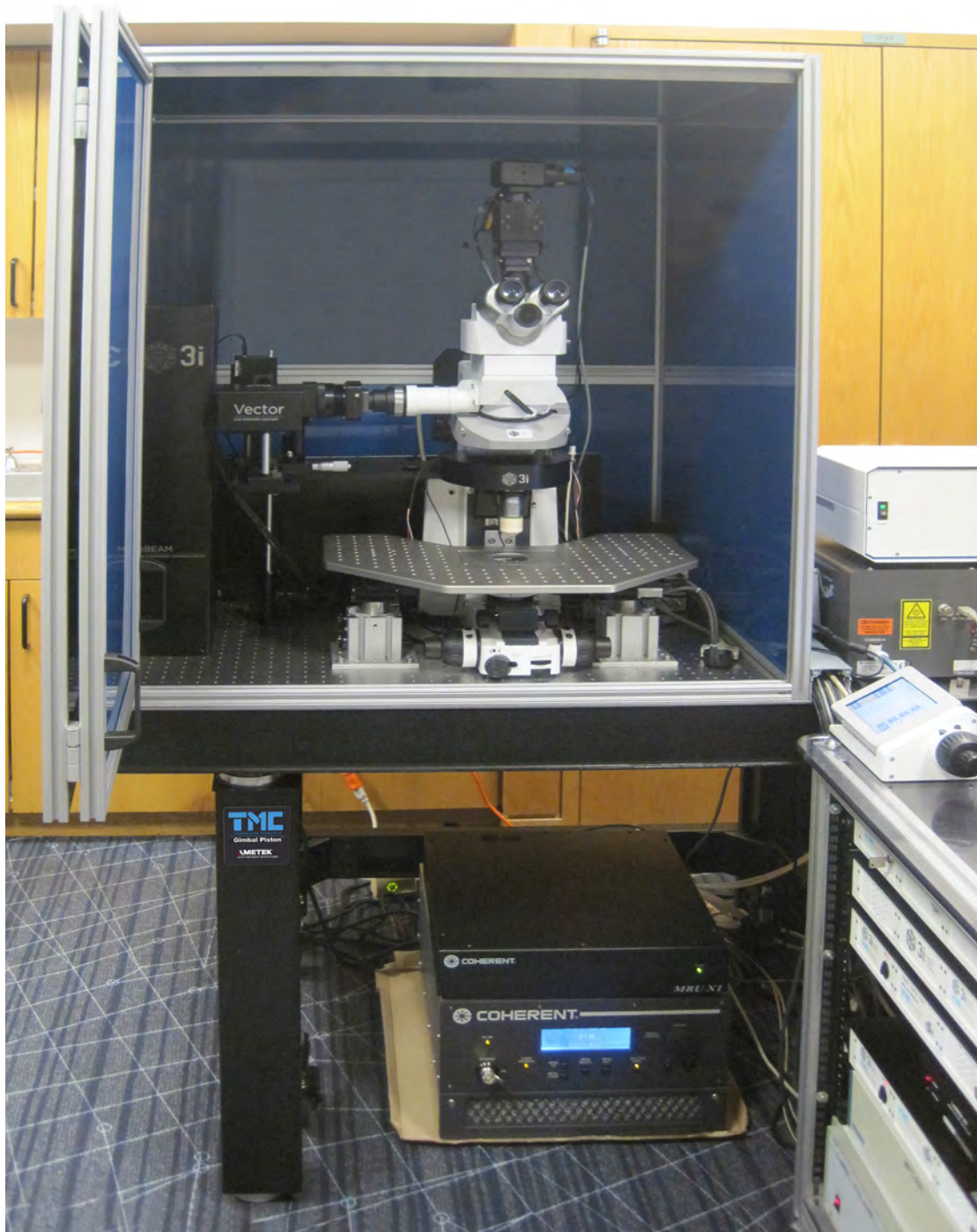
3i's (Intelligent Imaging Innovations) VIVO 2-Photon platform is a fixed stage upright instrument designed for high-speed multiphoton imaging of live animals and tissue. The system incorporates a tunable infrared ultrashort pulsed laser to provide multiphoton excitation and imaging of cellular activity deeper into tissue than more traditional microscopy techniques. Shown above is the TMC Micro-g® Lab Table 63-573.
