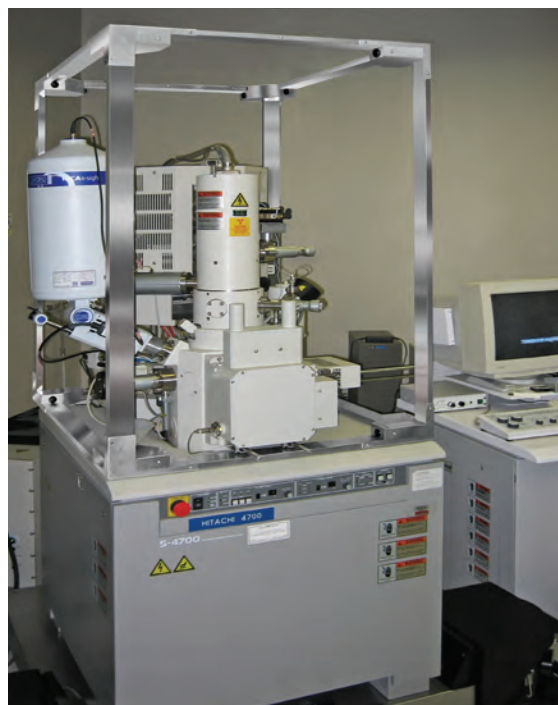
Mag-NetX™ System with Helmholtz coils mounted on a Hitachi S-4700 scanning electron microscope column.
