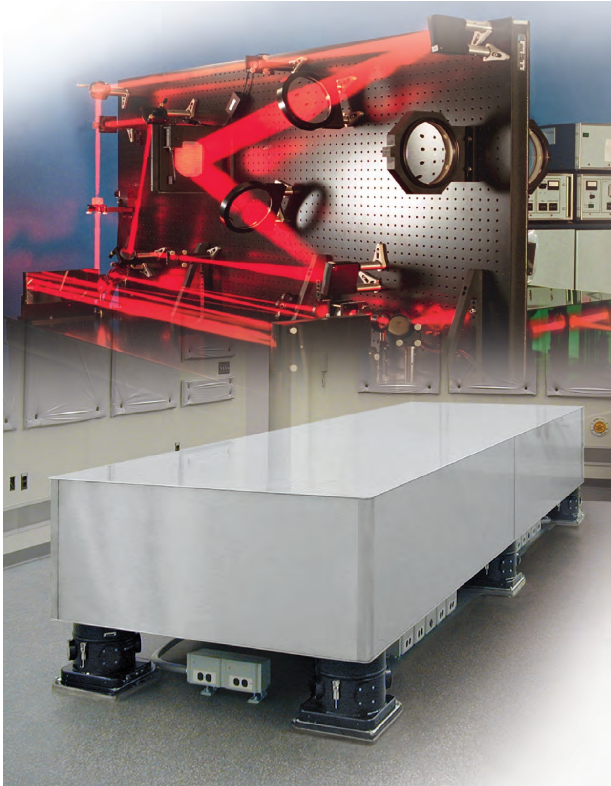
Top photo courtesy of MetroLaser; bottom, NASA Goddard's Advanced Interferometer and Metrology Lab (AIM) incorporates two 5 ft. x 16 ft. x 2 ft. Invar CleanTop® Optical Tops, each supported on a six-mount STACIS® active piezoelectric vibration cancellation system.
